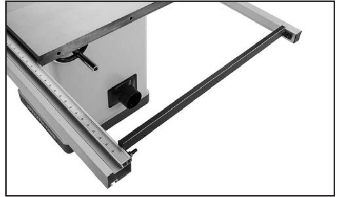
Figure 37. Fence rail brace installed.
